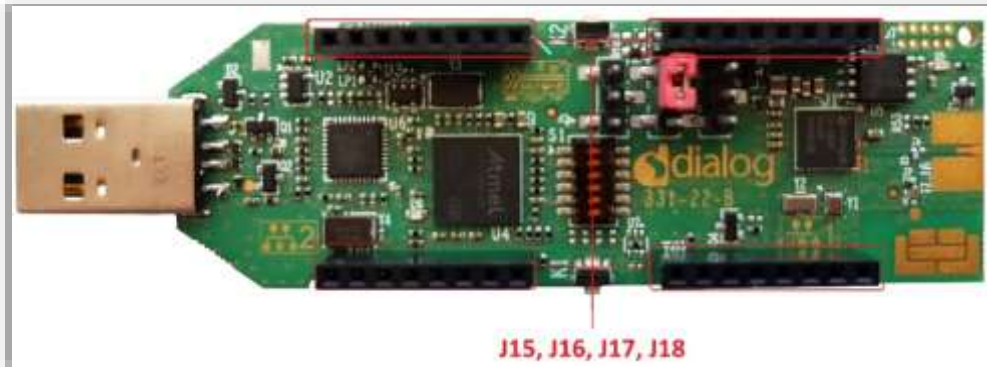
Figure 20: J15, J16, J17, and J18 Female Sockets (Must Be Soldered by Users)
