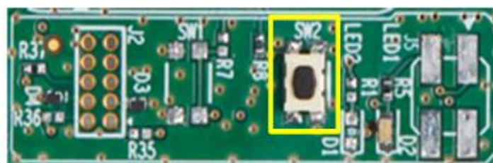
Figure 18. Default general purpose push button (SW2) on DA14535 SMARTBOND TINY™ MODULE DB
