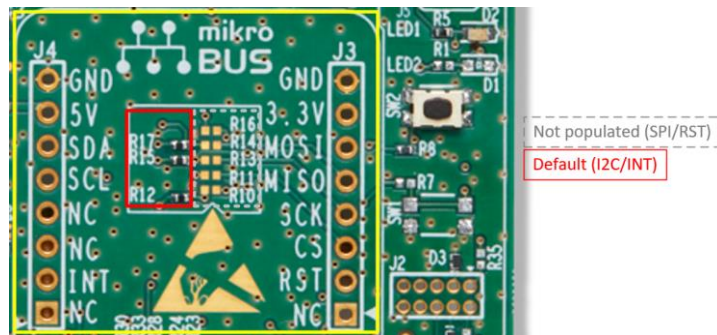
Figure 23. Default programming interface of MikroBUS™ module on DA14535 SMARTBOND TINY™ MODULE DB
