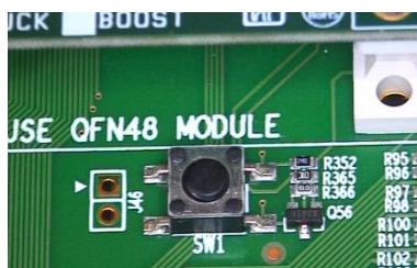
Figure 113. R365 (10 k \Omega ) added next to Reset button
