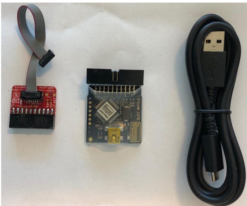
Figure 2: Segger J-Link Lite and 20-to-10 Pin Adapter with Cable
