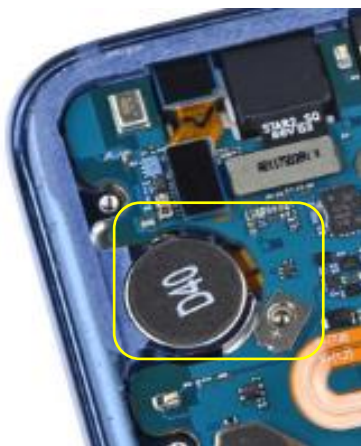
Figure 2: LRA Mounted in Mobile Phone
