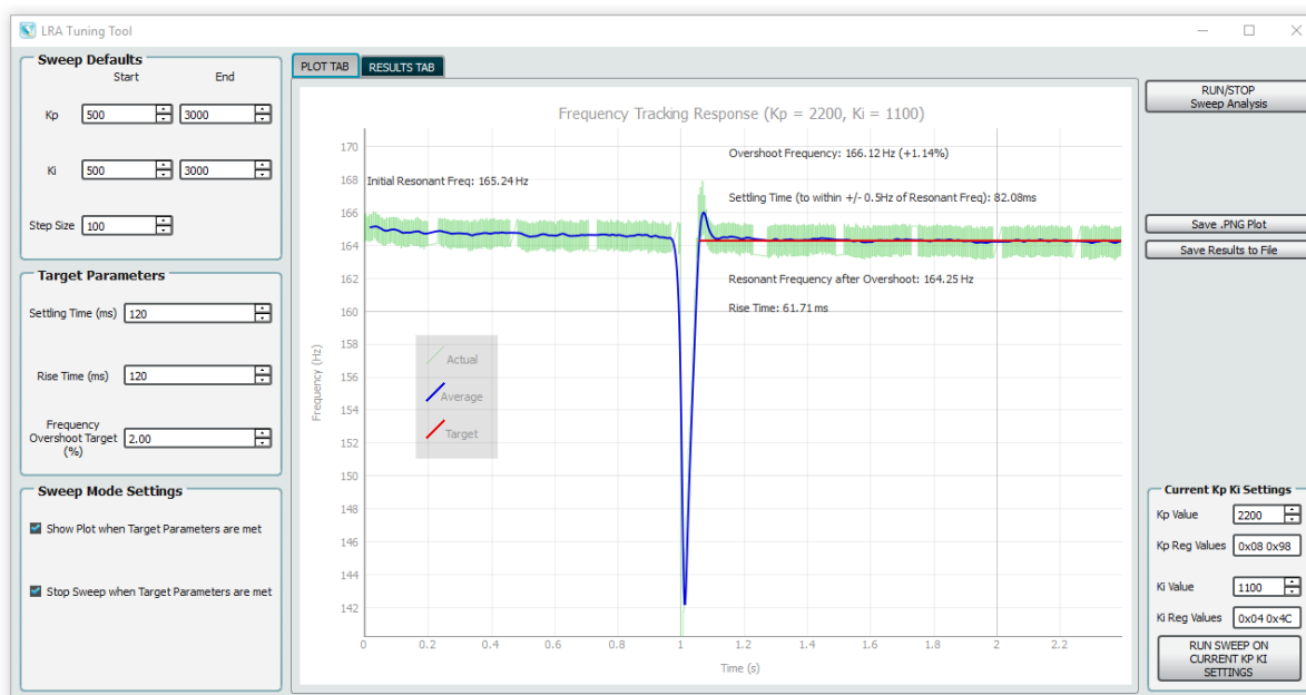
Figure 12: Good Frequency Tracking Settling Behavior; Good Loop Stability
