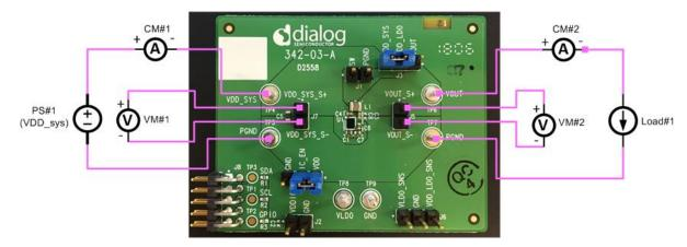
Figure 4: Recommended Setup for Buck Efficiency Measurement
