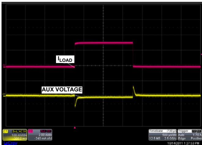
FIGURE 9. AUXILIARY VOLTAGE 3A LOAD TRANSIENT RESPONSE
