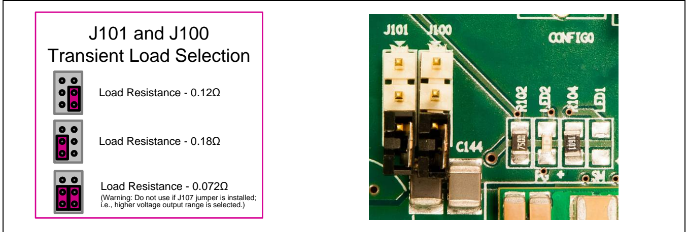
Figure 6.3 J100 and J101 – Transient Load Selection
