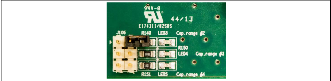
Figure 6.2 J106 - Output Capacitor Range Hardware Selection
