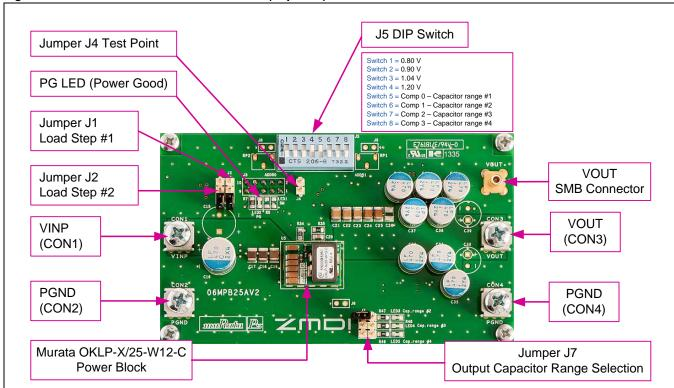
Figure 2.1 ZSPM8725-KIT Evaluation Board (Top Side)
