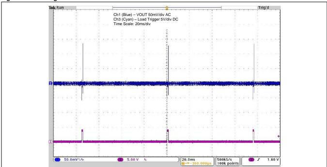
Figure 6.3 Timing for the On-Board Transient Loads
