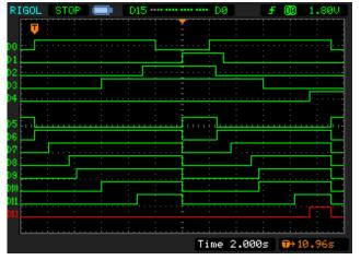
2. Reset function diagram, RESET\_1 and RESET\_2 are HIGH
