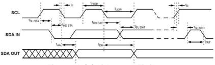
Figure 2. I2C Serial General Timing
