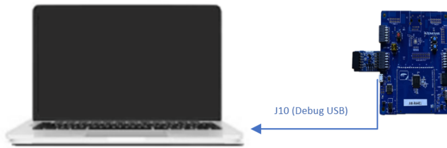
Figure 3. Connecting the AIK-RA4E1 Board to the Host PC via USB Debug Port
