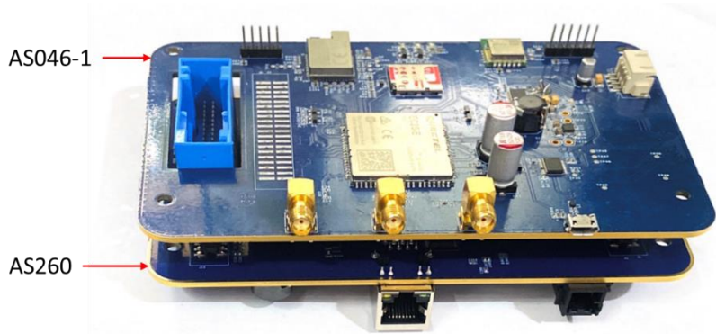
Figure 4-10 AS049-1-REIN-WCU-V1 and AS260 stack up.
