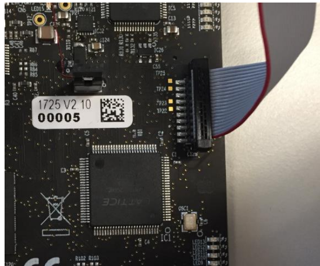
Figure 2-3: I-Jet Debugger connection
