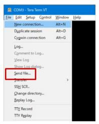
2. Select "Flash\_Writer\_SCIF\_RZG2L\_SMARC\_PMIC\_DDR4\_2GB\_1PCS.mot" and then click "Open" button. The image will be sent to the board via the serial connection.
