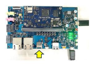
2. Turn on the board's power by pressing the power red button SW9. The settings of Terminal in this process are the same as in section 2.2.2.
