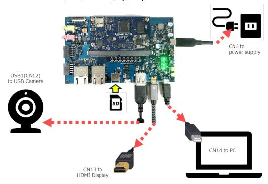
2. After EVK booting up, by the following command, the USB Camera Capture image which size of 1920×1080 will be displayed on the HDMI display.
