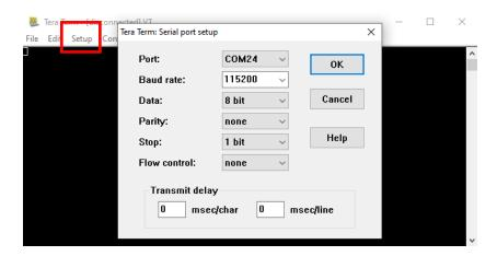
After selecting the serial port setup, press the blue button (RESET). Check that the message below is displayed on the console.
