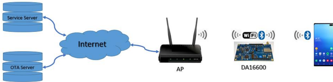
Figure 8. Diagram of provisioning through Bluetooth® LE
