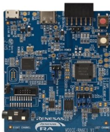
Figure 3. Voice Kit RA6E1 Board & USB Debug cable
