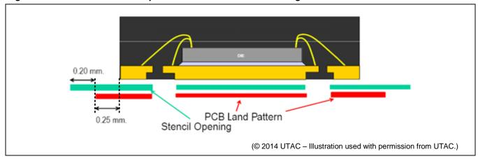
Figure 6.2 illustrates the recommended landing pattern for the ZSSC3018 QFN24 package.
