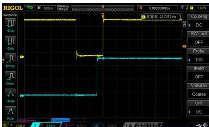
Figure 1. ACMP Output Glitch
