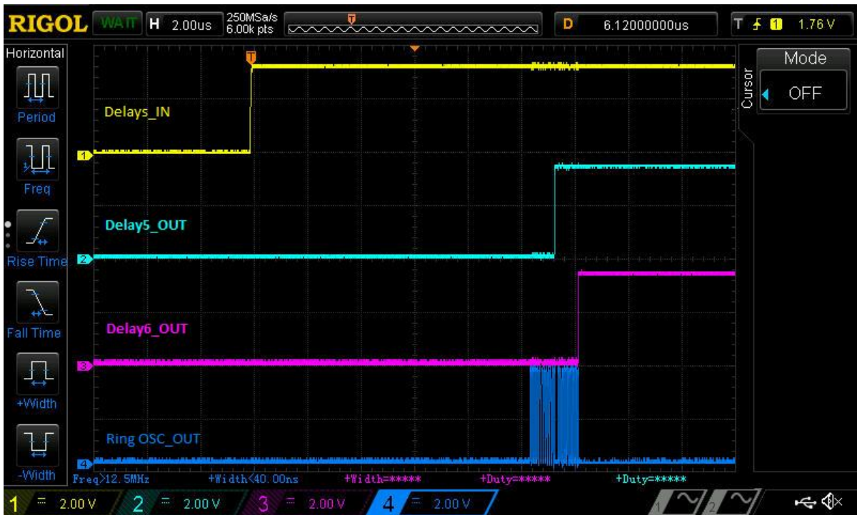
Figure 6. Ring OSC, DLY5 and DLY6 Waveform
