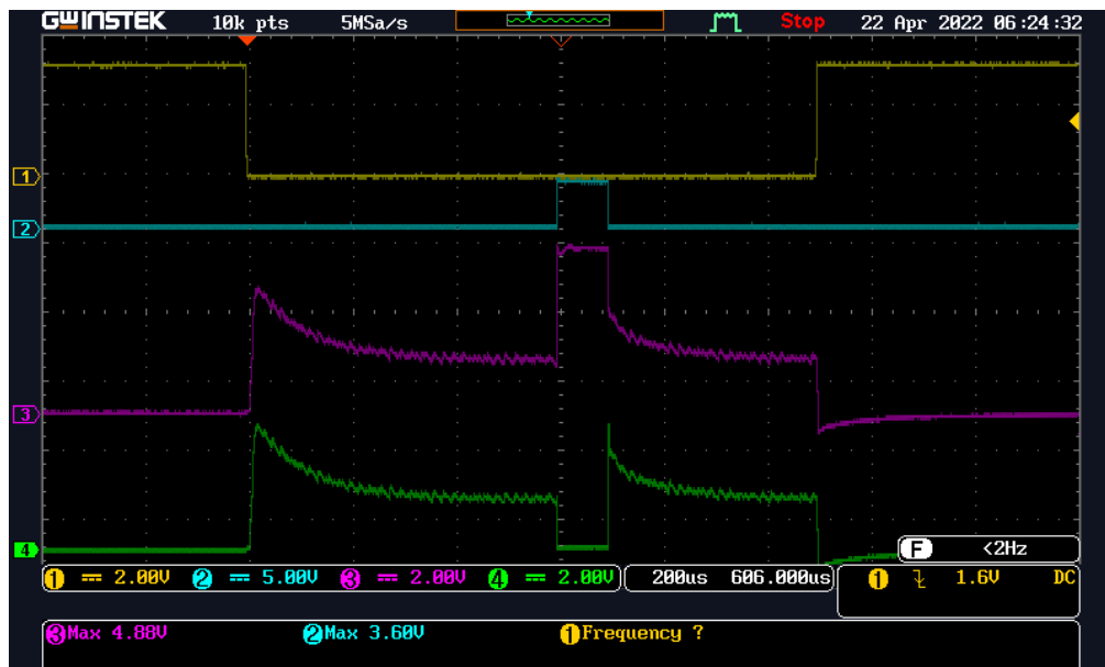
Figure 7 Glitch at HV_GPOx, decay = 0 (Fast decay)
