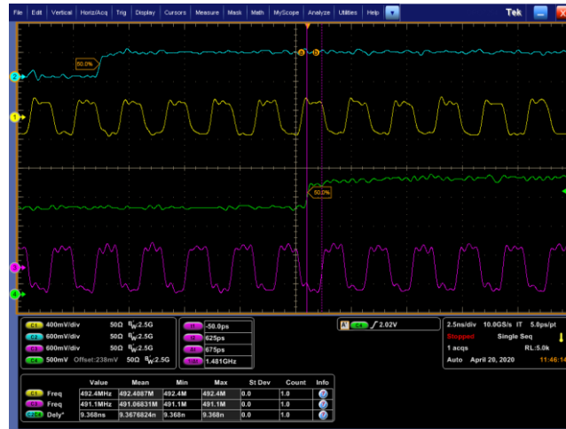
Figure 5. Zoom-In to Show 8V79S680 QREF-to-QCLK Phase Deterministic
