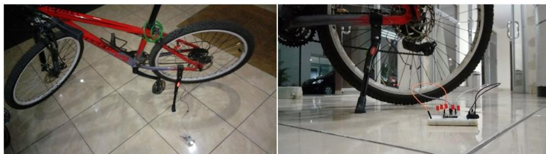
Figure 9: Magnet and Magnetic Switch Attached to Bicycle
