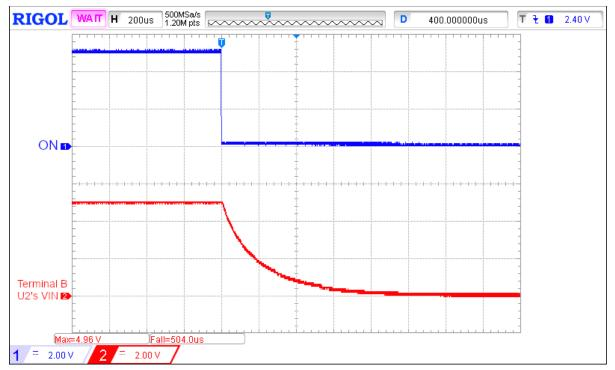
Figure 4. BLS Turn-OFF Operation for Two, Series-Connected SLG59M1558V GreenFET Load Switches for  $V_{IN(A)} = 5 V$ ,  $R_{LOAD} = 20 \Omega$ ,  $C_{LOAD} = 10 \mu F$
