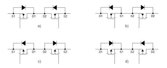
Figure 1. Common Configurations for BLS Realization
