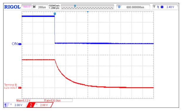
Figure 8. BLS Turn-OFF Operation Using a Pair of Series-Connected SLG59M1709V GreenFET Load Switches for  $V_{OUT(A)} = 5 \text{ V}$ ,  $R_{LOAD} = 20 \Omega$ ,  $C_{LOAD} = 10 \mu F$
