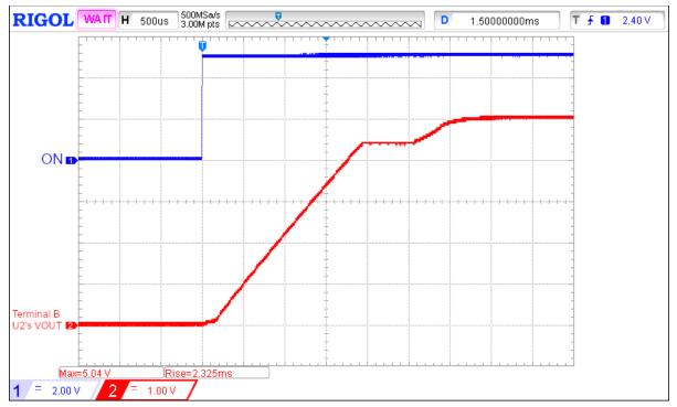
Figure 7. BLS Turn-ON Operation Using a Pair of Series-Connected SLG59M1709V GreenFET Load Switches for V<sub>OUT(A)</sub> = 5 V, R<sub>LOAD</sub> = 20 Ω, C<sub>LOAD</sub> = 10 μF
