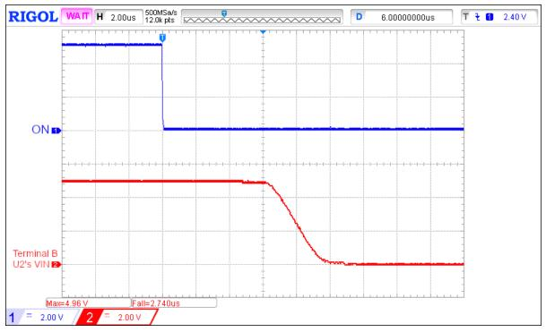
Figure 5. BLS Turn-OFF Operation for Two, Series-Connected SLG59M1558V GreenFET Load Switches for  $V_{IN(A)} = 5 V$ ,  $R_{LOAD} = 20 \Omega$ , no  $C_{LOAD}$
