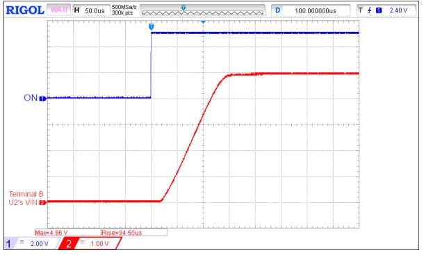
Figure 3. BLS Turn-ON Operation for Two, Series-Connected SLG59M1558V GreenFET Load Switches for  $V_{IN(A)} = 5 V$ ,  $R_{LOAD} = 20 \Omega$ ,  $C_{LOAD} = 10 \mu F$
