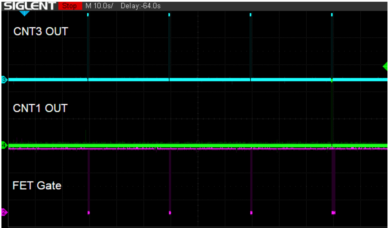
Figure 3 Waveforms that Illustrate Work of Toothbrush during One Brushing Session
