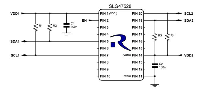
Figure 2: Bidirectional I<sup>2</sup>C Level Shifter Circuit
