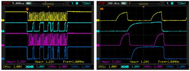
Figure 7: Low to High Voltage Level Shifting
