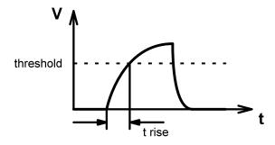
Figure 4: Pin Voltage Rise Time Definition
