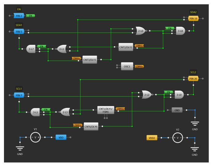
Figure 3: Bidirectional I<sup>2</sup>C Level Shifter Design
