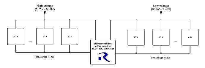
Figure 1: Typical Block Diagram for Bidirectional Level Shifting
