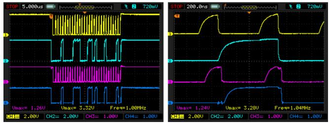
Figure 5: High to Low Voltage Level Shifting
