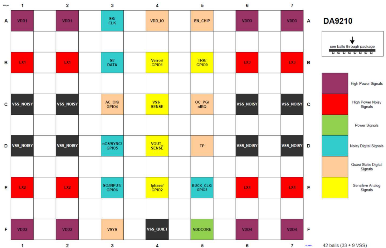
Figure 2: DA9210 42VF-BGA ball map
