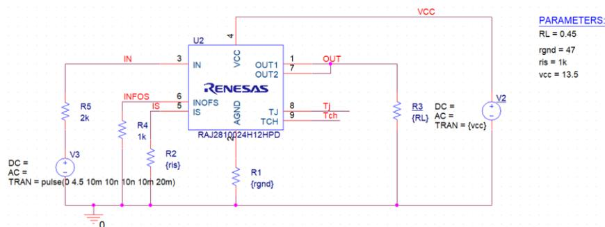
Figure.7 Simulation Circuit
