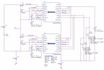
Figure.9 Simulation Circuit (Half-bridge operation)
