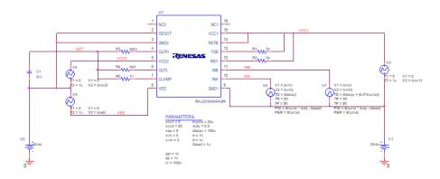
Figure.7 Simulation Circuit (Basic characteristics)
