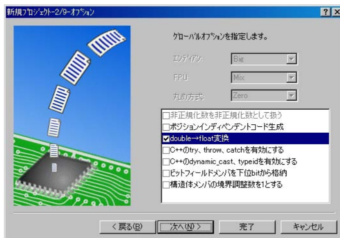
図 6.1 単精度の指定方法 (SH-1, SH-2, SH-2E, SH-2A, SH2-DSP, SH-3, SH3-DSP, SH4AL-DSP)
