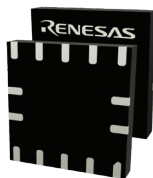
3.0 mm x 3.0 mm 14-pin FCQFN 0.65 mm pitch
