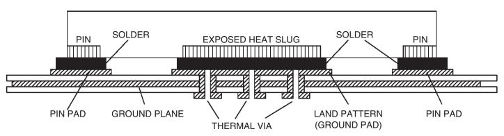
Figure 7. P.C. Assembly for Exposed Pad Thermal Release Path - Side View (drawing not to scale)
