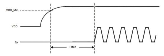
Figure 1. Stabilization Time (T<sub>stab</sub>)
