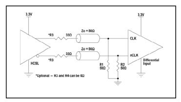
Figure 5C. CLK/nCLK Input Driven by a 3.3V HCSL Driver
