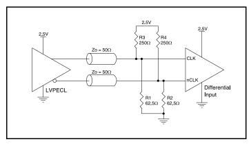
Figure 6B. CLKx/nCLKx Input Driven by a 2.5V LVPECL Driver
