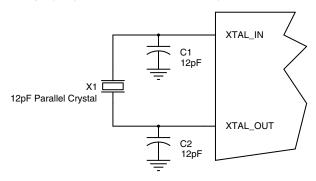
Figure 3. Crystal Input Interface
