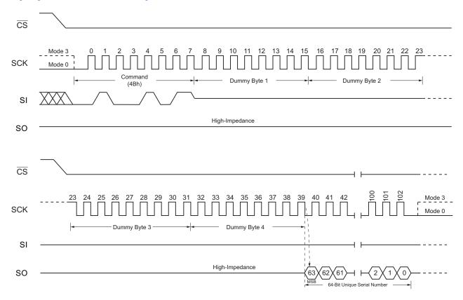
Figure 27. Read Unique ID Timing (SPI Mode)
