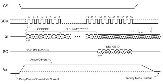
Figure 41. Resume from Deep Power-Down and Read Device ID
