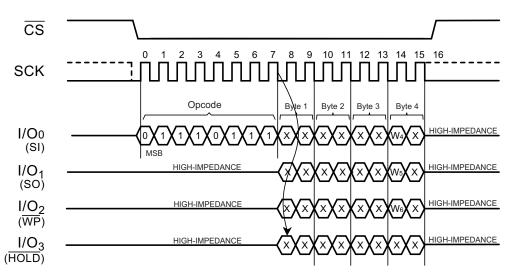
Figure 13. Set Burst with Wrap Timing (SPI Mode)
