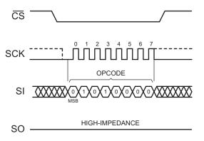
Figure 34. Write Enable for Volatile Status Register
