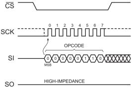
Figure 24. Write Enable Sequence Diagram
