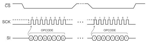
Figure 26. Enable Reset (66h) and Reset Device (99h) Command Timing (SPI Mode)
