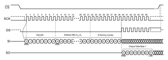
Figure 16. Read Serial Flash Discoverable Parameter Command Sequence Diagram
