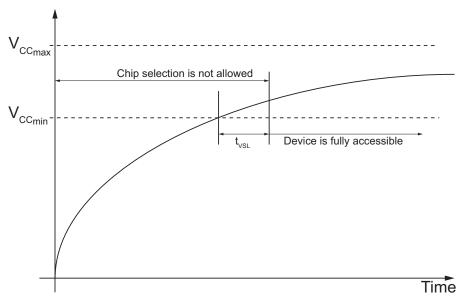
Figure 42. Power-Up Timing and Voltage Levels
