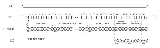
Figure 7. Dual-Output Fast Read Array
