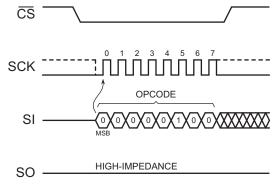
Figure 25. Write Disable Sequence Diagram
