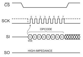
Figure 21. Chip Erase Sequence Diagram
