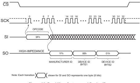
Figure 35. Read Manufacturer and Device ID
