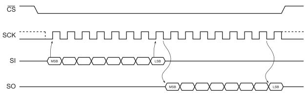
Figure 4. SPI Mode 0 and 3
