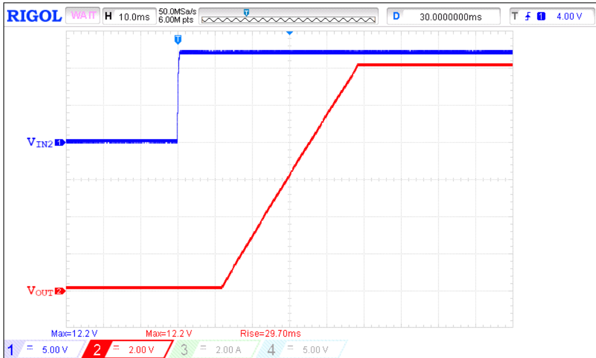
Figure 5. Typical Turn ON operation waveform for V_{IN2} = 12\text{ V} , C_{SS} = 220\text{ nF} , R_{LOAD} = 100\ \Omega , C_{LOAD} = 2\ \mu\text{F}
