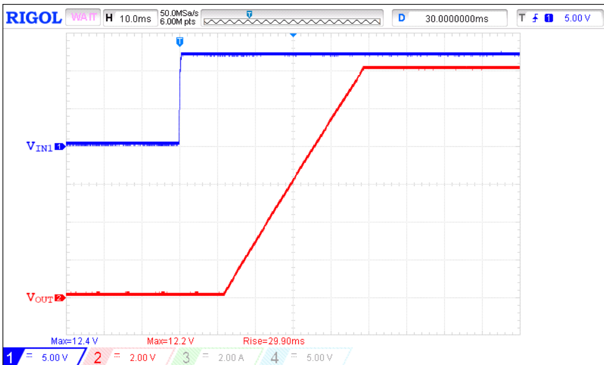
Figure 2. Typical Turn ON operation waveform for V_{IN1} = 12\text{ V} , C_{SS} = 220\text{ nF} , R_{LOAD} = 100\ \Omega , C_{LOAD} = 2\ \mu\text{F}
