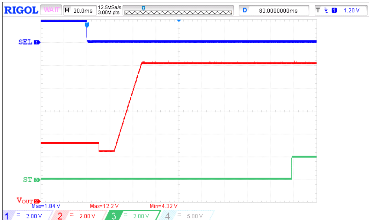
Figure 8. Switchover operation waveform for V_{IN1} = 12\text{ V} , V_{IN2} = 5\text{ V} , C_{SS} = 220\text{ nF} , PR = 0\text{ V} , SEL = \text{High} \rightarrow \text{Low} , R_{LOAD} = 100\ \Omega , C_{LOAD} = 2\ \mu\text{F}
