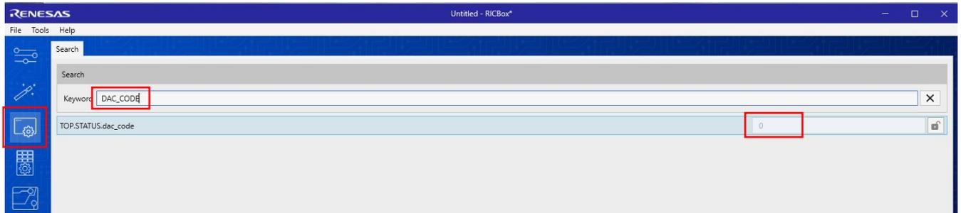
Figure 18. Activate DCB\_CAL and Check DAC\_CODE Value
