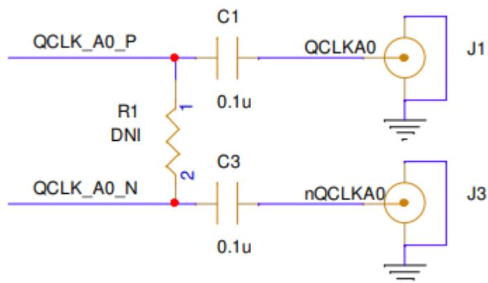
Figure 11. Output Clock AC-Coupling
