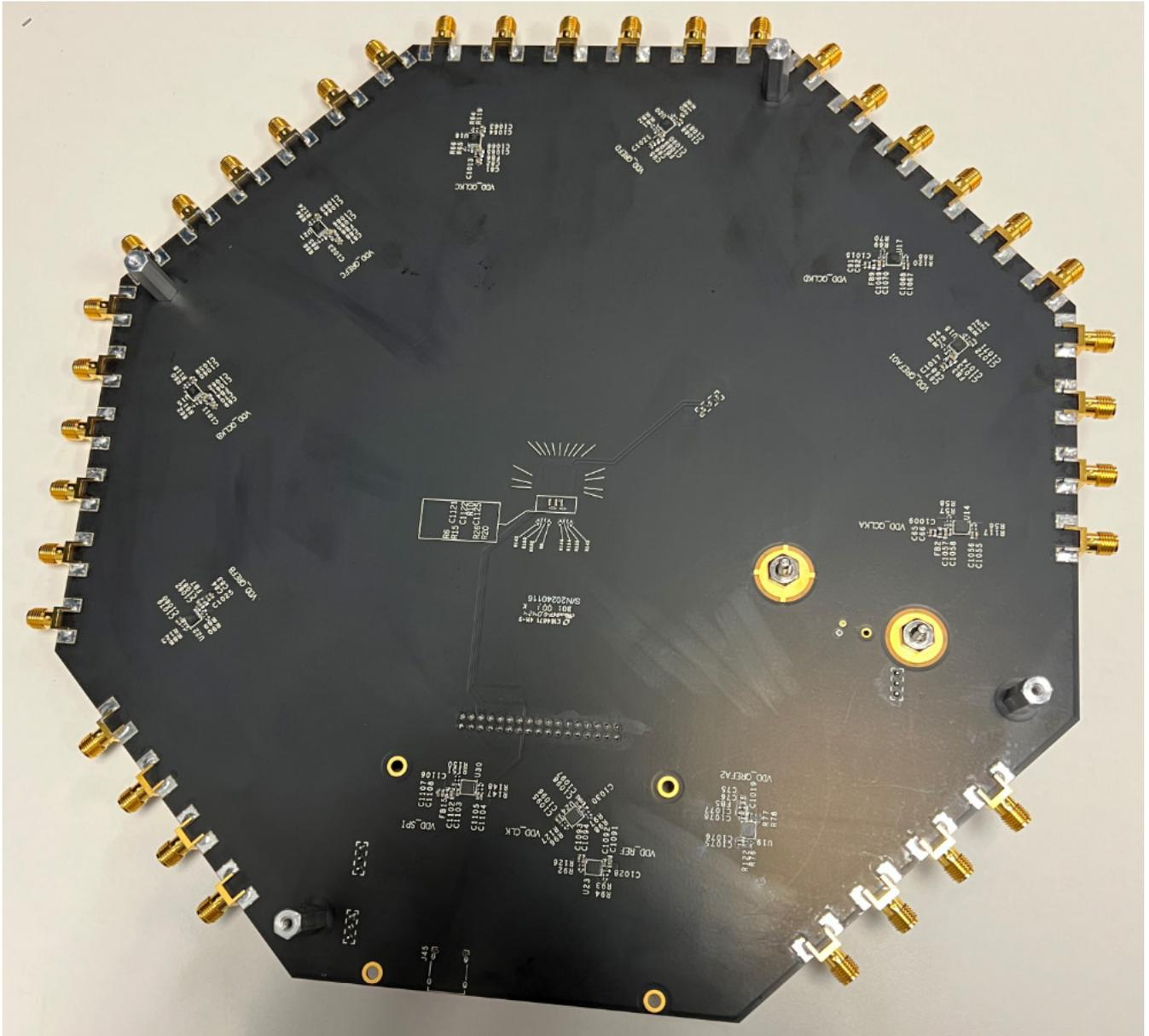
Figure 26. 8V79S680/8V79S683/RC18016 Evaluation Board (bottom)
