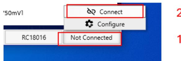
Figure 22. Connect to the Device in RICBox
