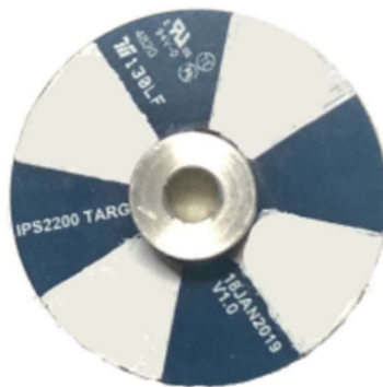
Figure 23. Reflector Board, Mounted onto Rotor
