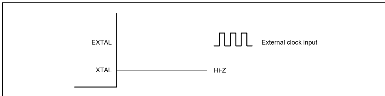
Figure 8.5 Equivalent circuit for external clock
