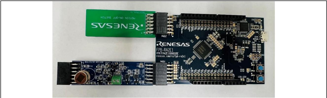
**Figure 48. Button board as well as QCIOT-14 board connected to FPB-RA2E1 board**
