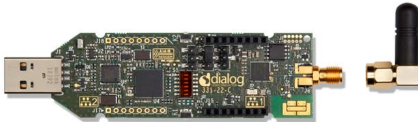
Figure 23: DA14695 USB Kit HW Components with External Antenna
