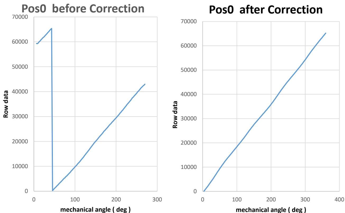
Figure 5. Example of Pos0 Values before and after Zero-Offset Correction
