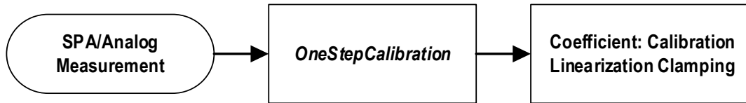
Figure 11. Inputs and Outputs for OneStepCalibration
