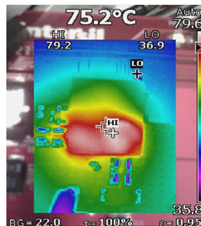
Figure 15. Thermal Image, 12V_{IN} to 1V_{OUT} , I_{OUT} = 25A , T_A = 25°C , f_{SW} = 550kHz , No Air Flow
