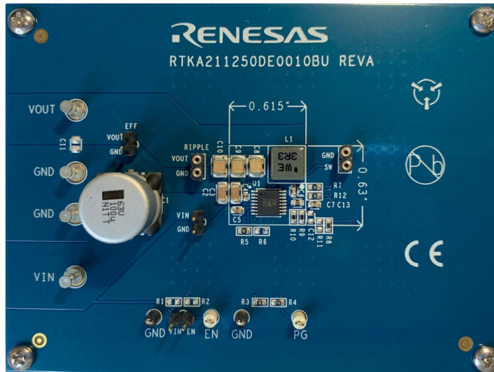
Figure 3. RTKA211250DE0010BU Evaluation Board (Top)
