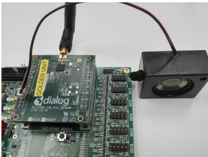
Figure 174: Speaker Connection for Audio Test.
