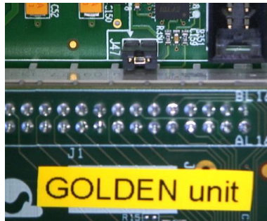
Figure 158: Jumper J47 Added Next to Golden Unit Socket
