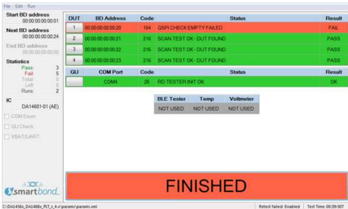
Figure 119: GUI PLT tests finished
