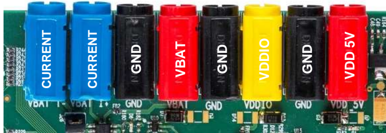
Figure 4: PLT hardware power connections
