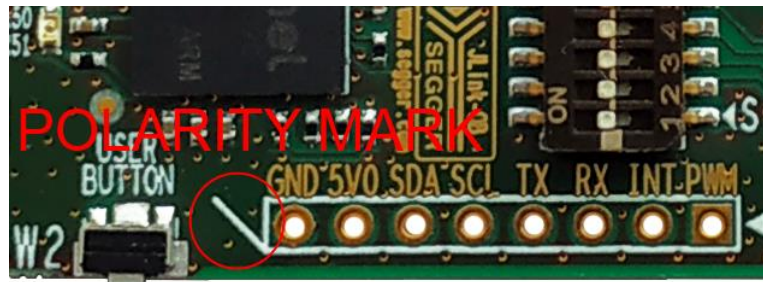
Figure 18. Guides for proper mikroBus™ click board insertion
