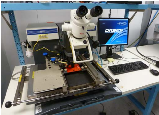
FIGURE 8. REWORK STATION WITH THERMAL PROFILE CONTROL
