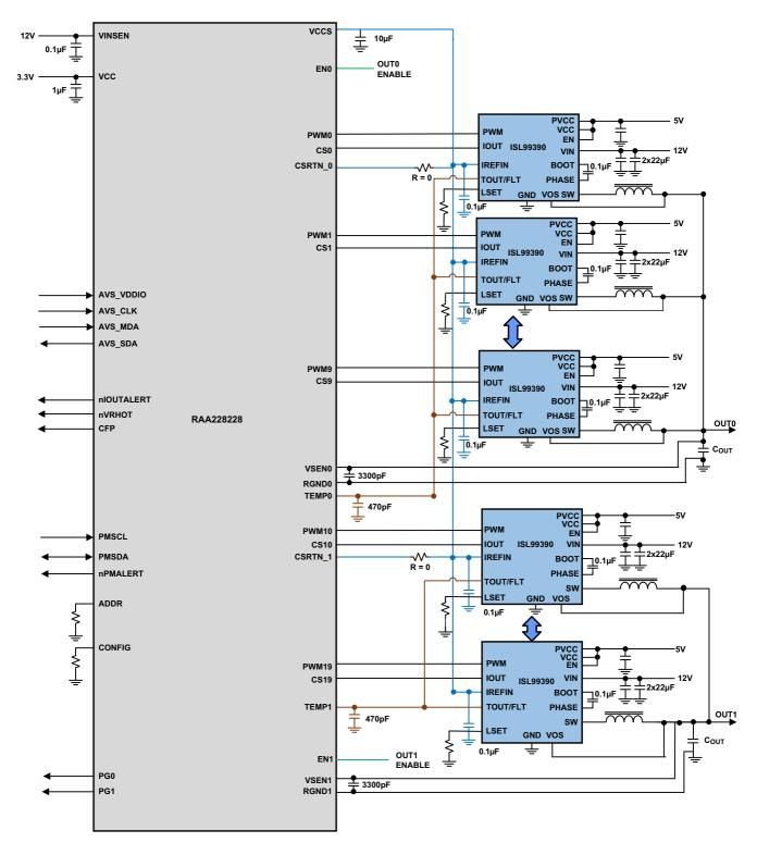
Figure 1. 10+10 Smart Power Stage
