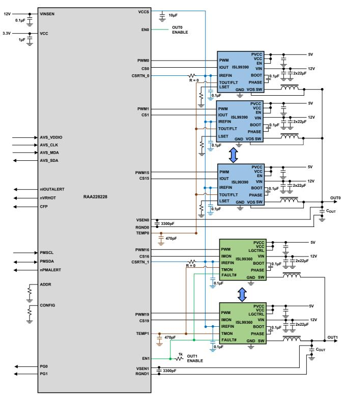
Figure 2. 16+4 Smart Power Stage
