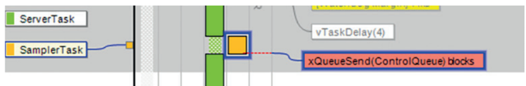
Figure 2. SamplerTask blocks on a send-to-queue operation.
