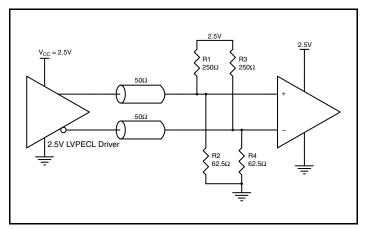
Figure 4A. 2.5V LVPECL Driver Termination Example
