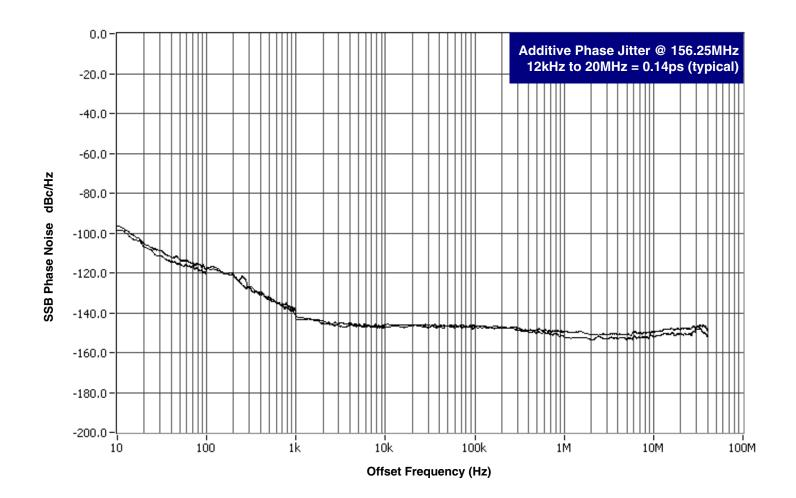
As with most timing specifications, phase noise measurements has issues relating to the limitations of the equipment. Often the noise floor of the equipment is higher than the noise floor of the device. This is illustrated above. The device meets the noise floor of what is shown, but can actually be lower. The phase noise is dependent on the input source and measurement equipment.
