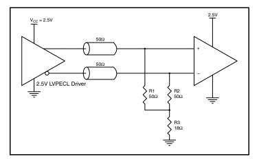
Figure 4B. 2.5V LVPECL Driver Termination Example
