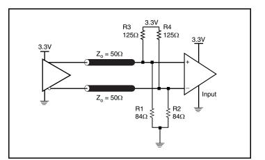
Figure 3B. 3.3V LVPECL Output Termination
