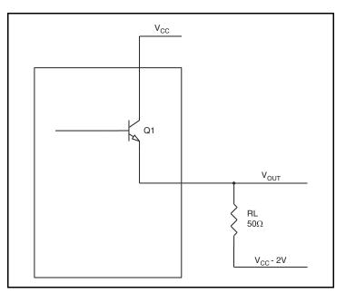
Figure 5. LVPECL Driver Circuit and Termination
