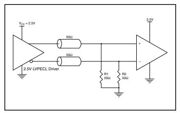
Figure 4C. 2.5V LVPECL Driver Termination Example
