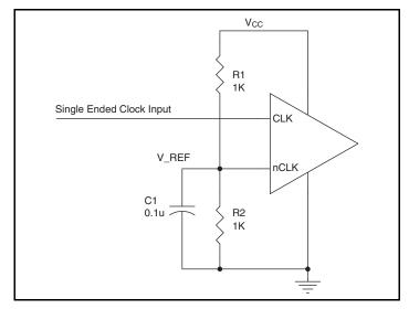
Figure 1. Single-Ended Signal Driving Differential Input
