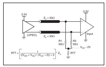
Figure 3A. 3.3V LVPECL Output Termination
