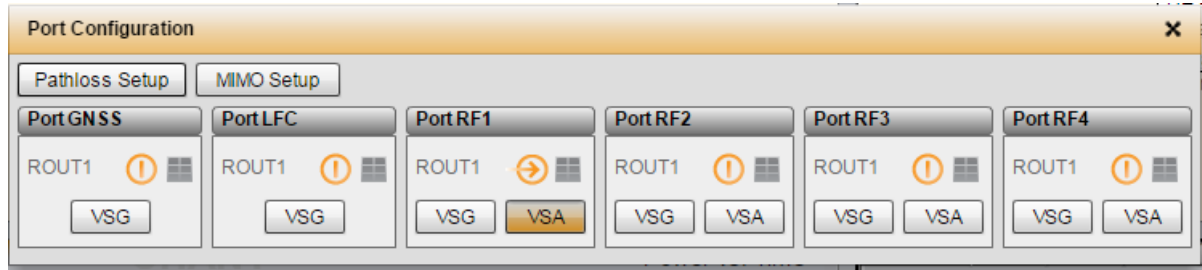
Figure 18: IQxel Port Configuration – using Port RF1 for VSA
