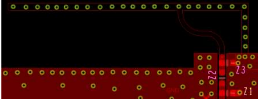
Figure 26: RF matching circuit must be placed as close as possible to the antenna
