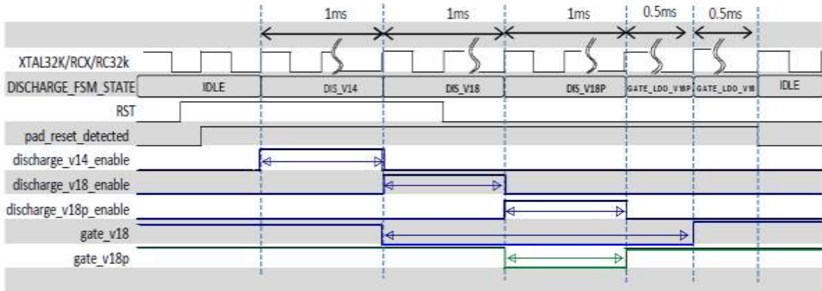
Figure 10: Discharging rails FSM timing
